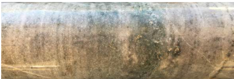
MIDD007 60m quartzite with disseminated pyrite and chlorite alteration
