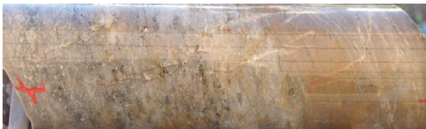
MIDD006 82.8m dissem. pyrite and chalcopyrite in conglomerate 0.13% Co, 0.20% Cu, 0.06 g/t Au
