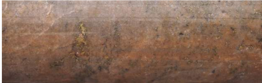
MIDD005 66.1m disseminated chalcopyrite and minor pyrrhotite 0.08% Co, 0.63% Cu, 0.12 g/t Au
