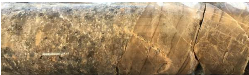
MIDD001 106m contact between conglomerate and laminated sandy sediments
