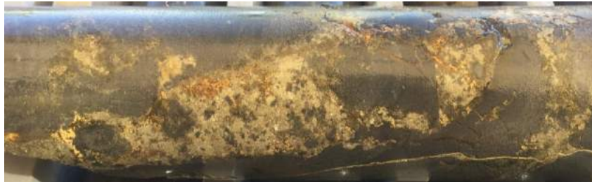
MIDD004 31.8m coarse sulphides in graphitic shale, 0.05% Co, 0.12% Cu, 0.01 g/t Au
