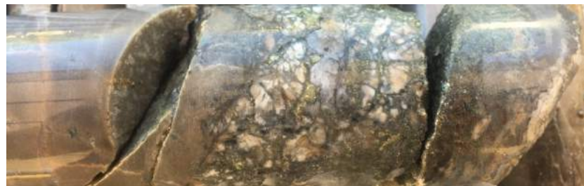
MIDD008 54.1m chalcopyrite breccia vein in quartzite 0.02% Co, 0.61% Cu, 0.07 g/t Au
