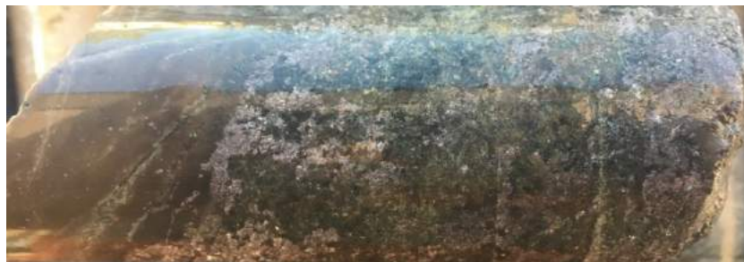
MIDD010 41m cobaltite chlorite mineralisation in quartzite 1.85% Co, 0.18% Cu, 0.42 g/t Au
