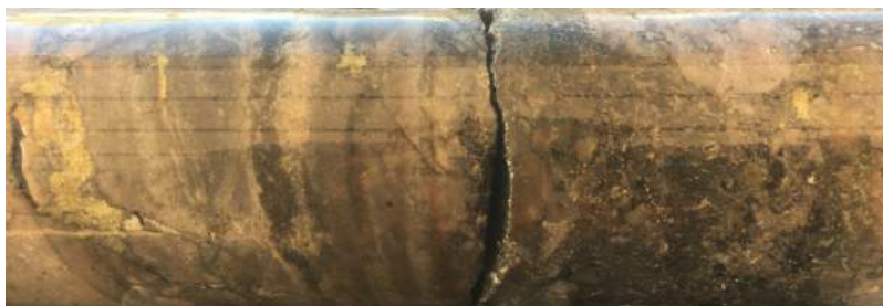
MIDD010 50.8m chalcopyrite pyrite vein in quartzite 0.14% Co, 0.52% Cu, 1.24 g/t Au
