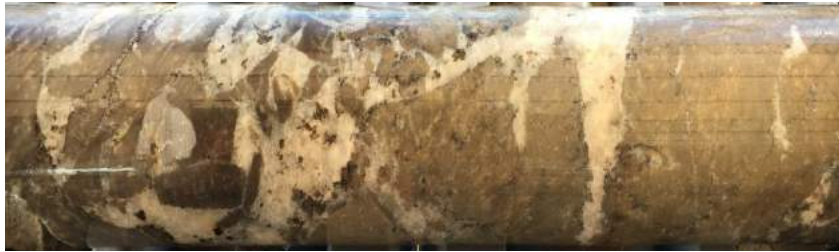
MIDD001 54.9m quartzite 0.03% Co, 0.19% Cu, 0.75 g/t Au
