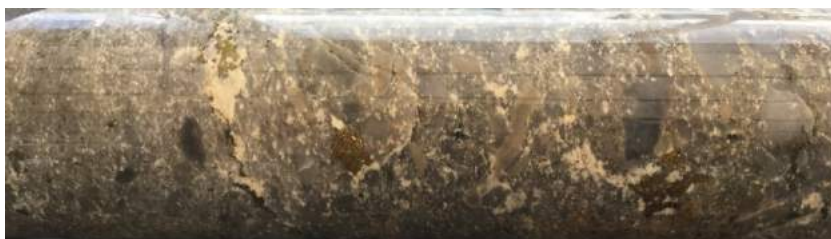
MIDD003 91.7m coarse pyrite in conglomeratic unit, 0.07% Co, 0.32% Cu, 0.09 g/t Au
