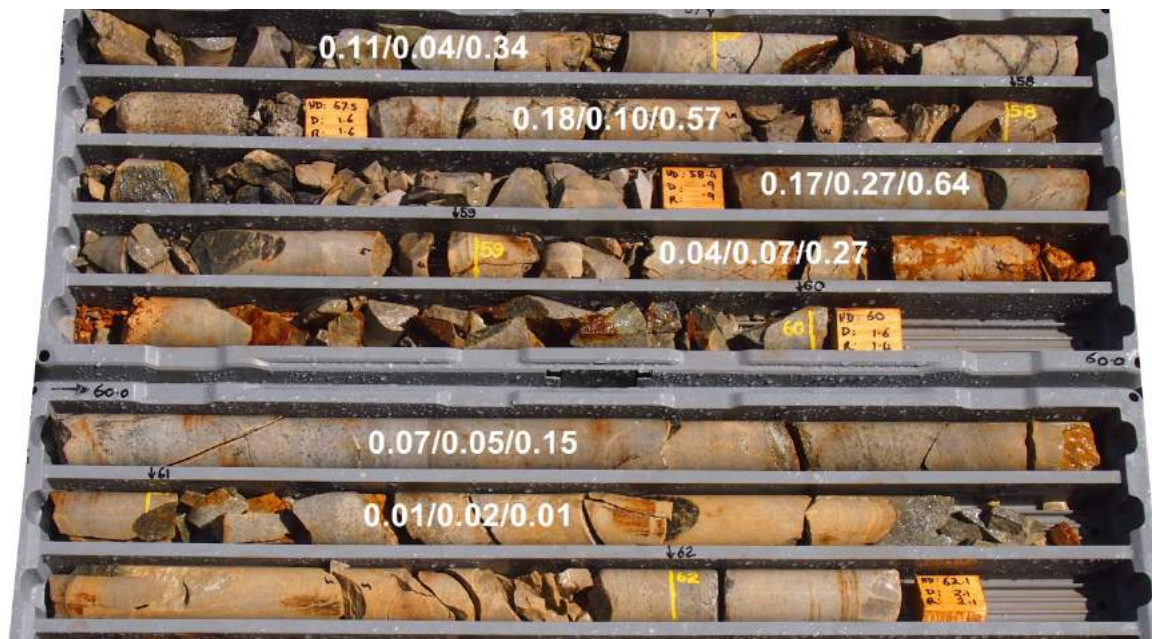
Plate 10-5 Photograph of mineralised intersection in MIDD005 with Au g/t / Co % / Cu % assays
