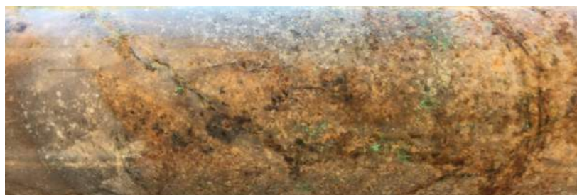
MIDD009 41.2m malachite bearing quartzite 0.08% Co, 0.74% Cu, 0.25 g/t Au
