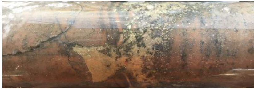
MIDD009 70.5m chalcopyrite pyrite vein in quartzite 0.42% Co, 0.83% Cu, 0.25 g/t Au
