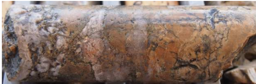
MIDD005 53.5m quartz coarse pyrite vein in quartzite 0.05% Co, 0.69% Cu, 0.38 g/t Au
